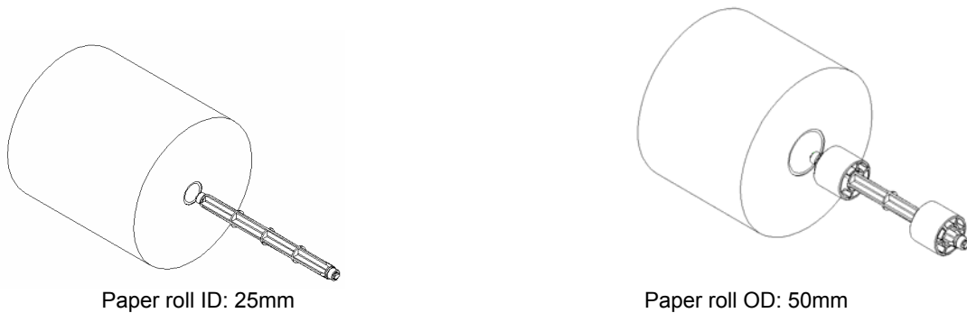
Figure 4.9 Explanation for installing paper roll holding shaft
